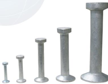
Manufactured in high quality, galvanized steel, the Lifting Pin Anchor provides a disc-shaped foot embedded in the concrete engaged by the Pin Insert Lifting Eye. Safe Working Loads displayed in below chart apply to loading in any direction.
